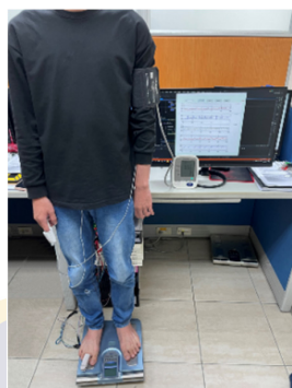
Figure 5. A subject stands on the commercial weight scale. The finger of right hand and toe of right foot wears the PPG probes. The cuff of blood pressure monitor is wrapped on the left hand. Lead I ECG is measured.
